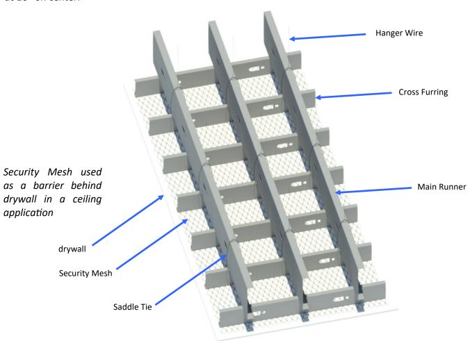
Material: Type II, Class 1 - Carbon Steel - Mesh, complying to ASTM F1267 Sheet Size: 48" x 96"
