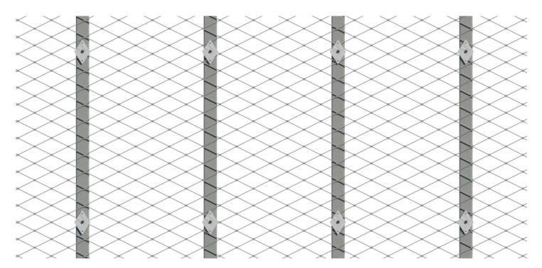
DCM Security Mesh Clips are installed 12" on center vertically on framing members. Studs are typically spaced at 16" on center.
